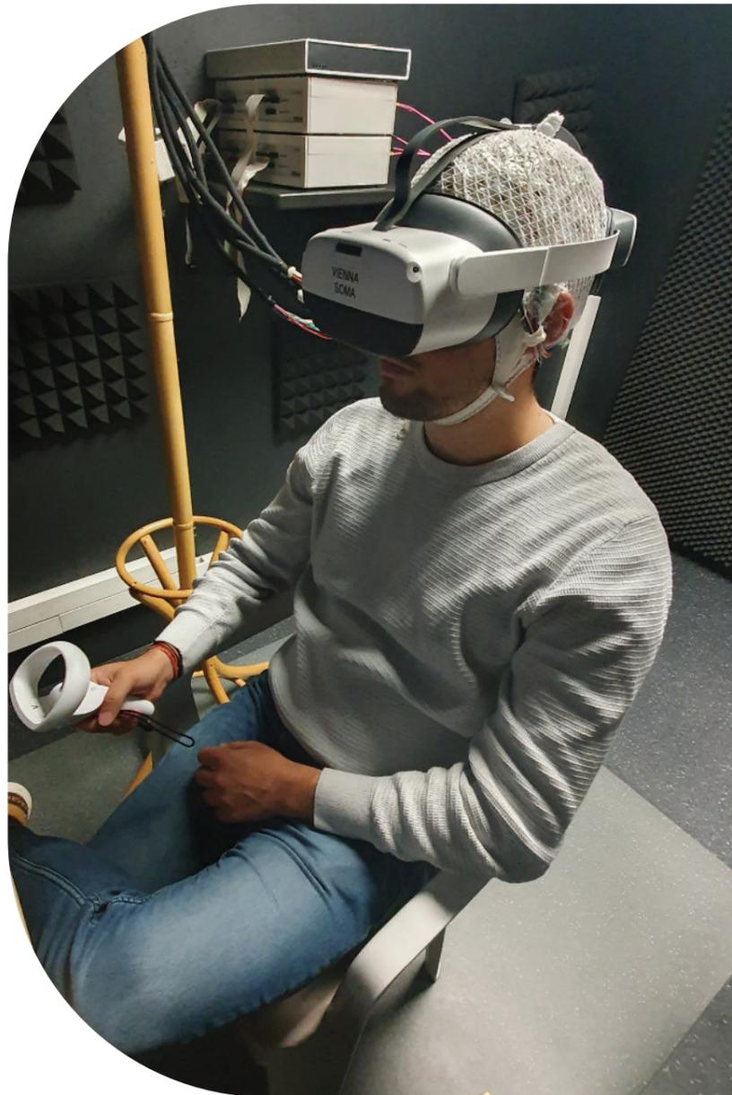
The PICO Neo 3 Pro Eye is an advanced standalone virtual reality (VR) headset with integrated eye-tracking technology, designed for professional applications in research, training, and enterprise environments. Building upon PICO's VR platform, the Neo 3 Pro Eye combines high-resolution displays with precise eye-tracking capabilities to enable sophisticated gaze-based interactions and cognitive research applications.
